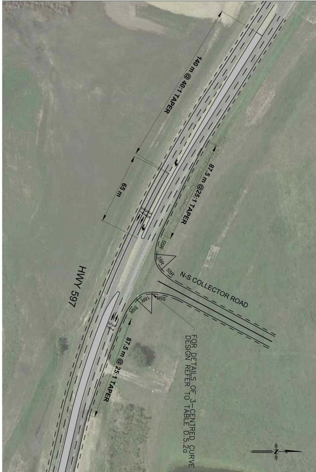
Figure 12. AT Preferred Intersection Improvement Concept Plan (South Access)
